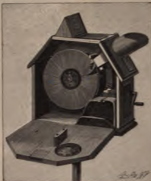
INTERIOR OF THE "MUTOSCOPE."
