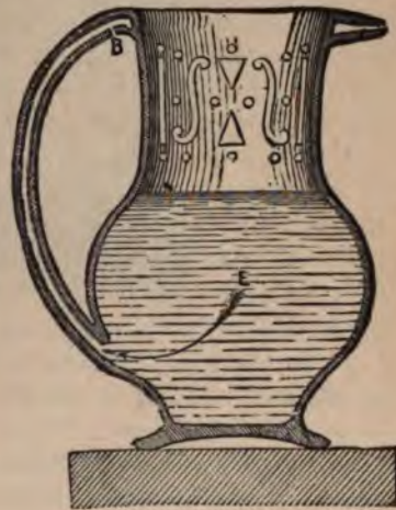
FIG. 6.—SECTION OF A MAGICAL PITCHER.
