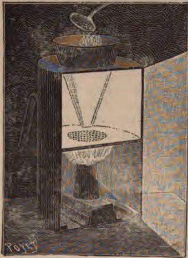
APPARATUS FOR PRODUCING LIGHTNING.
