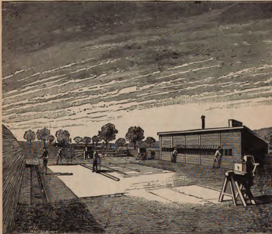
FIG. 1.—ARRANGEMENTS ADOPTED BY MR. MUYBRIDGE IN HIS EXPERIMENTS ON THE GAITS OF A HORSE.
